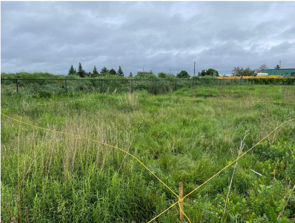
Appendix 2: 10m x 10m grid was set up using stakes and rope
